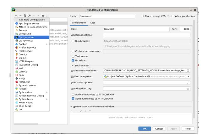
**Hint:** Be careful with the property called *No reload*: It prevents the server from being reloaded live if you modify files. This allows the existing debugger breakpoints to persist, when they normally would be discarded upon reloading the server.
